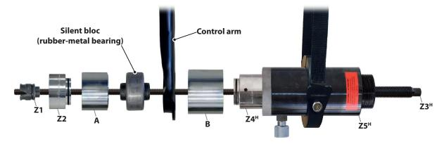
1. Assemble the silent bloc tool as shown and attach it to the control arm with the new silent bloc in the correct position.
