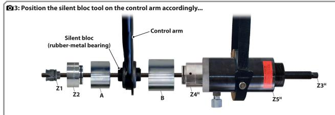
1. Assemble the silent bloc tool as shown and position it correctly on the silent bloc or control arm.
