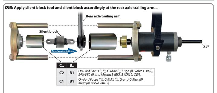
**1.** Compile the suitable silent block tool depending on the vehicle and apply it in the correct position on the rear axle trailing arm according to the direction of installation of the silent block.
