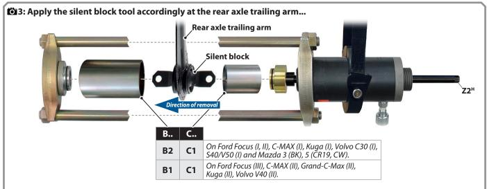
**1.** Compile the suitable silent block tool depending on the vehicle and apply it in the correct position on the rear axle trailing arm according to the direction of removal of the silent block.
