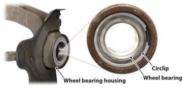
**4.** Mount the wheel bearing circlip on the wheel bearing housing with a suitable tool according to the manufacturer's specifications.
