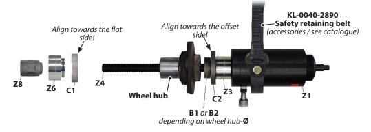
(i) The safety retaining belt - **KL-0040-2890** available as *accessory*, enables the wheel bearing tool to be secured to the vehicle to prevent it from falling down and being hurled around.
