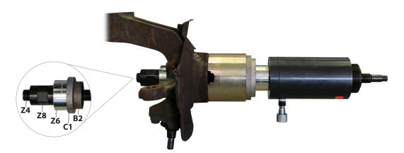
**3.** Apply the wheel bearing tool in the correct position on the wheel bearing housing, as shown, and secure with the clamping nut **[Z8]**. At the same time, pay attention that the centring ring **[B2]** sits neatly in the wheel bearing.
