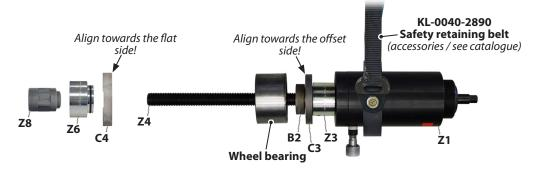
(i) The safety retaining belt - **KL-0040-2890** available as *accessory*, enables the wheel bearing tool to be secured to the vehicle to prevent it from falling down and being hurled around.
