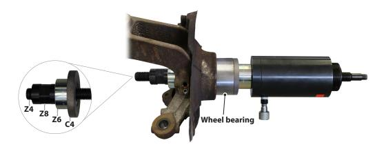
**2.** Apply wheel bearing tool together with the wheel bearing in the correct position on the wheel bearing housing, as shown, and secure with the clamping nut **[Z8]**. At the same time, pay attention that the centring ring **[B2]** sits neatly in the wheel bearing.
