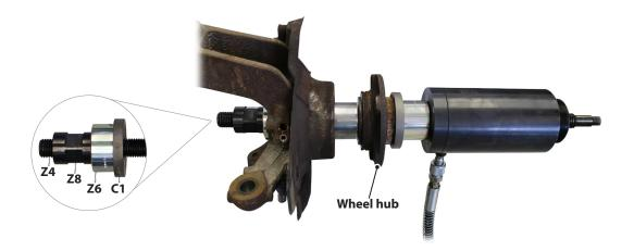
**2.** Apply the wheel bearing tool together with the wheel hub in the correct position on the wheel bearing housing, as shown, and secure with the clamping nut **[Z8]**. At the same time, pay attention that the centring ring **[B1]** or, depending on the wheel hub Ø, **[B2]**, sits neatly in the wheel hub.
