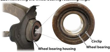
**1.** Remove the wheel bearing retaining ring on the wheel bearing housing using a suitable tool.
