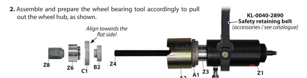
(i) The safety retaining belt - **KL-0040-2890** available as *accessory*, enables the wheel bearing tool to be secured to the vehicle to prevent it from falling down and being hurled around.
